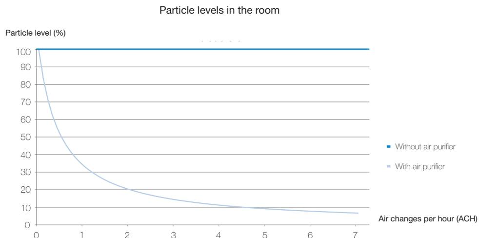
The graph shows that the indoor air quality is shown to reduce the particle levels by approximately 60% with 1 ACH. It is also shown that the more ACH in the room, the lower is the particle level. With 5 ACH the particle level is down 90% compared to without an air purifier in the room.
